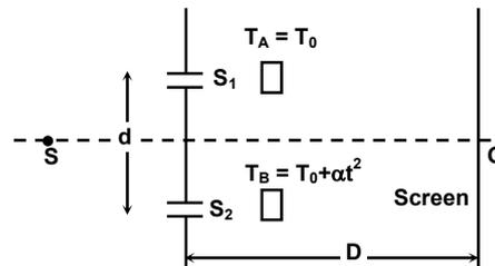
13. Two transparent slabs having equal thickness 0.45 mm and refractive indices 1.40 & 1.42 are pasted on the two slits of a double slit apparatus. The separation of slits equals 1 mm. Wavelength of light used equals 600 nm. The screen  $S$  is placed at a distance 1 m from the plane of the slits. Find the position(s) of first
